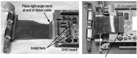
Installed ribbon cable/bracket assembly
