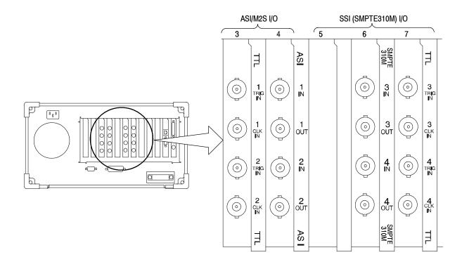
Figure 2-6: Rear-panel configuration with ASI/M2S (Option AS) and SSI (Option SS) interfaces installed
