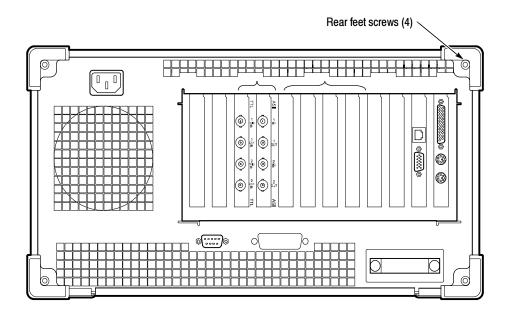
Figure 6-13: Removing the cabinet feet
