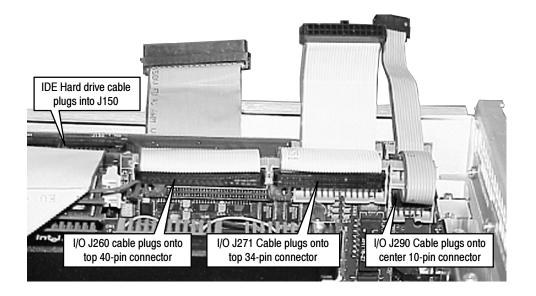
Figure 6-42: Processor I/O board to Controller board interconnections - top connectors
