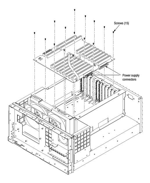
Figure 6-46: Backplane orientation and screw locations
