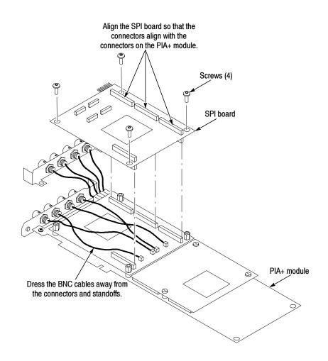
Figure 6-24: Installing the SPI board on the PIA+ module
