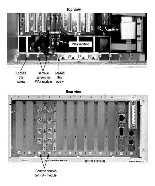
Figure 4-5: Removing the PIA+ module
