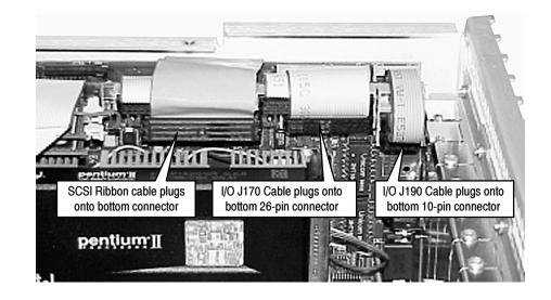
Figure 6-43: Processor I/O board to Controller board interconnections - bottom connectors
