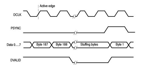
Figure 1-2: Parallel data timing, 188-byte packets
