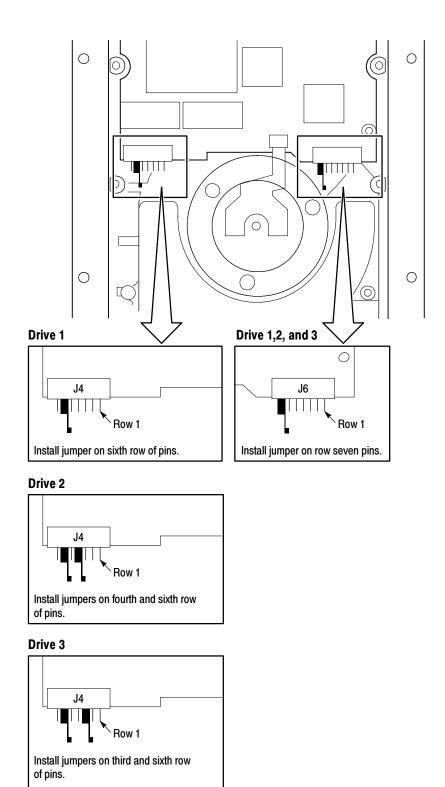
Figure 6-48: Configuring the SCSI drive jumpers
