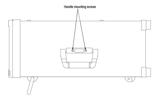
Figure 4-1: Removing the right-side handle screws
