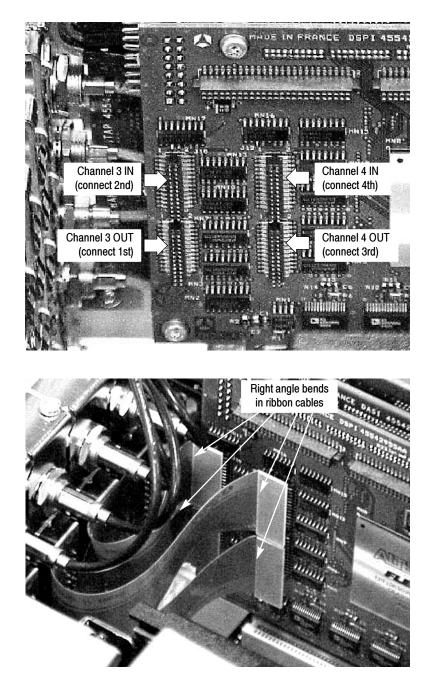
Figure 6-26: Connecting the ribbon cables on the SPI board
