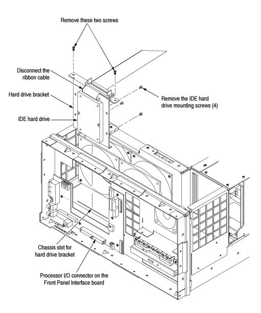
Figure 6-37: Removing the IDE hard drive
