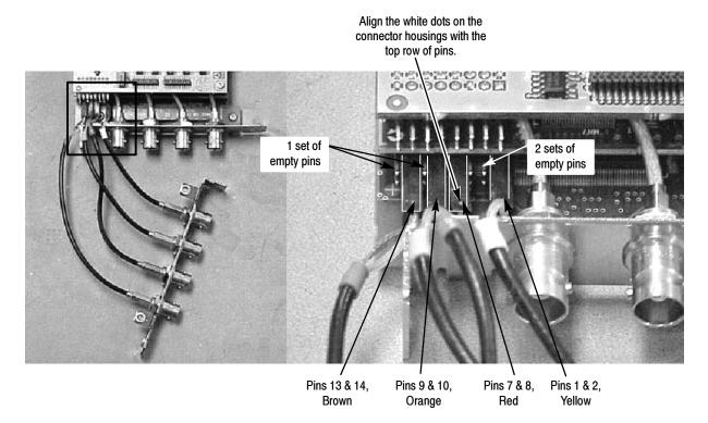
Figure 6-16: Clock and trigger cable connections for the ASI or SSI board on the PIA+ module
