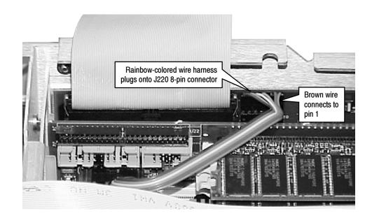
Figure 6-45: Location of J220 connections and wiring orientation
