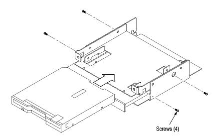
Figure 6-32: Chassis screw locations for the floppy disk drive
