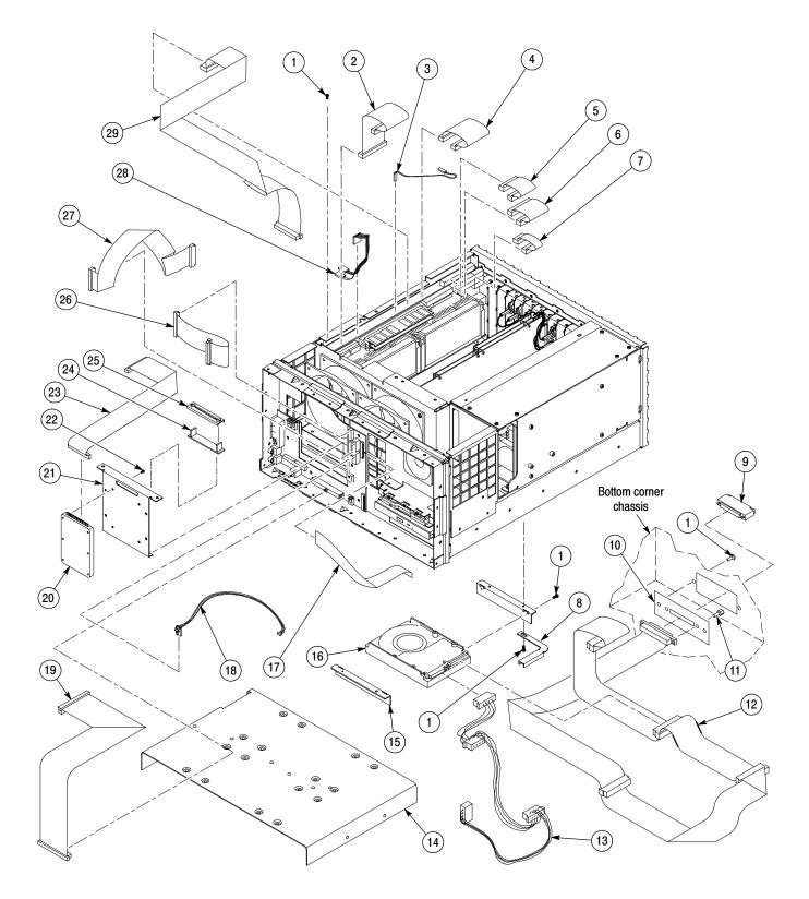
Figure 10-3: Cables and hard drives
