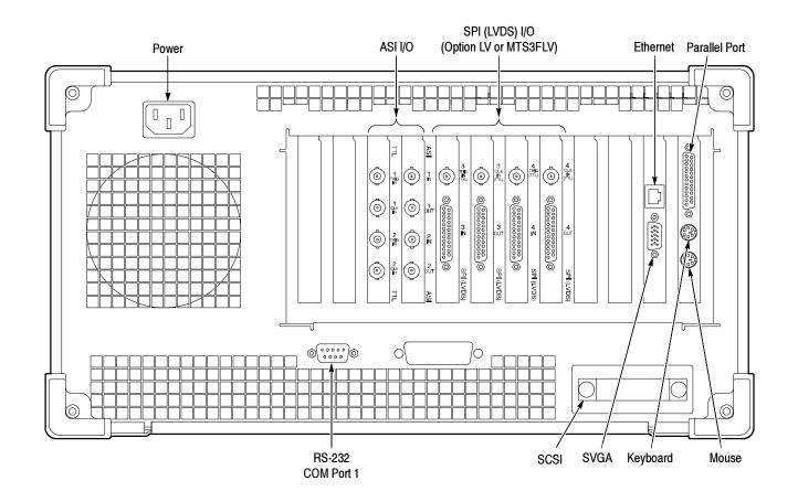
Figure 2-1: Typical MTS300 test system rear panel connectors
