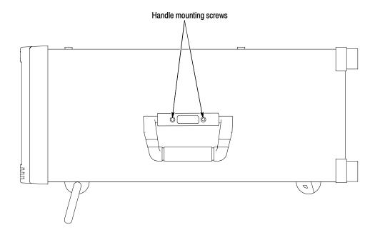
Figure 6-12: Removing the cabinet handle
