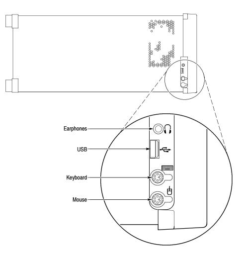
Figure 2-2: Keyboard and mouse alternative connections
