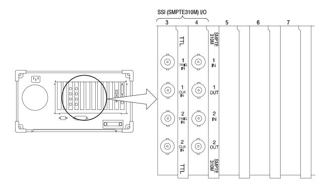
Figure 2-9: Rear-panel configuration with one SSI (Option SS) interface installed
