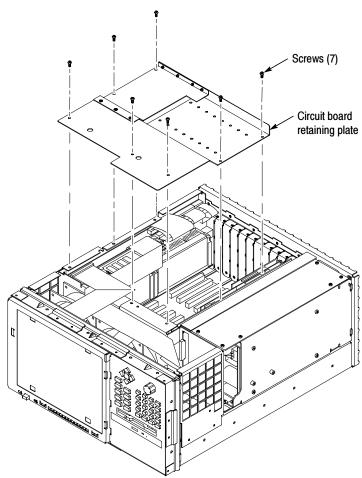
Figure 4-3: Removing the circuit board retaining plate
