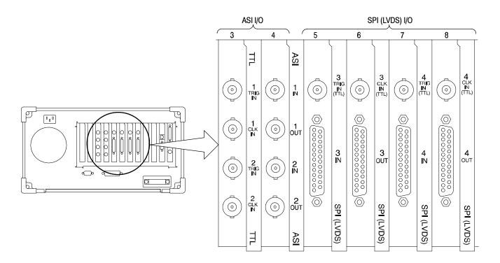
Figure 2-8: Rear-panel configuration with ASI/M2S (Option AS) and SPI (Option LV) interfaces installed
