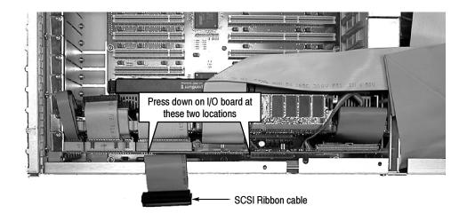
Figure 6-41: Installing the Processor I/O board into the backplane
