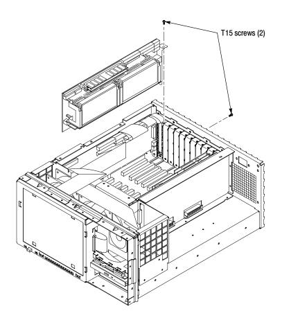
Figure 6-39: Controller board orientation and screw locations
