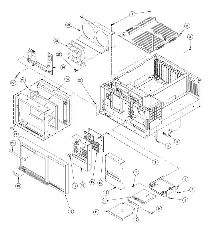
Figure 10-2: Front panel and associated parts, Backplane board, and disk drives
