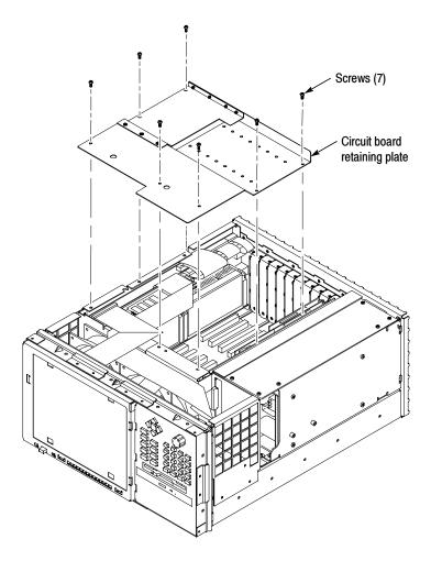
Figure 6-14: Circuit board retaining plate
