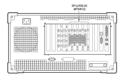
Figure 4-30: Rear panel connections for I/O #3 test procedure
