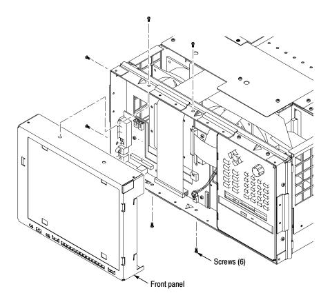
Figure 6-28: LCD Display assembly removal
