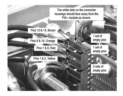
Figure 6-19: Clock and trigger cable connections on an additional SSI or ASI board
