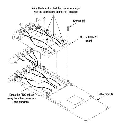
Figure 6-18: Installing an optional SSI or ASI board on the PIA+ module
