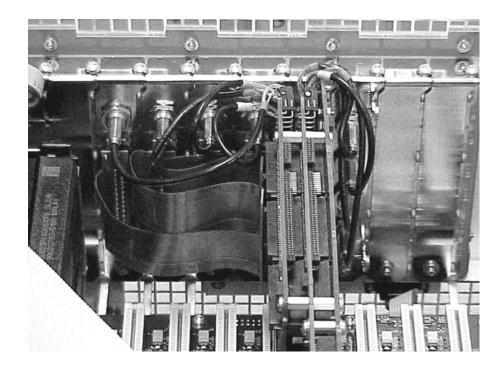
Figure 6-27: Optional SPI interface installation
