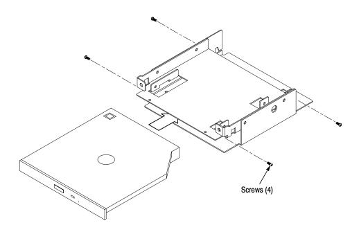
Figure 6-31: Chassis screw locations for CD drive
