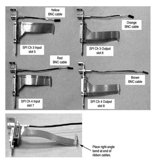
Figure 6-25: Assembling the SPI rear-panel brackets and cables
