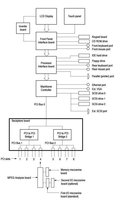
Figure 3-1: Mainframe simplified block diagram
