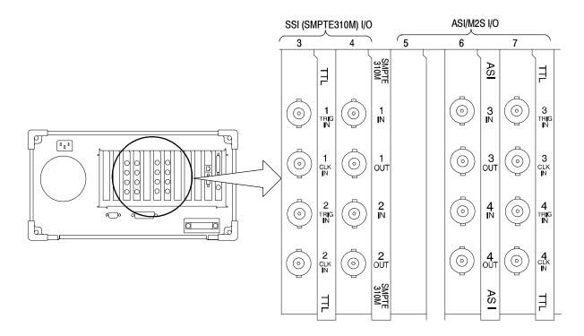
Figure 2-11: Rear-panel configuration with SSI (Option SS) and ASI/M2S (MTS3FAS) interfaces installed
