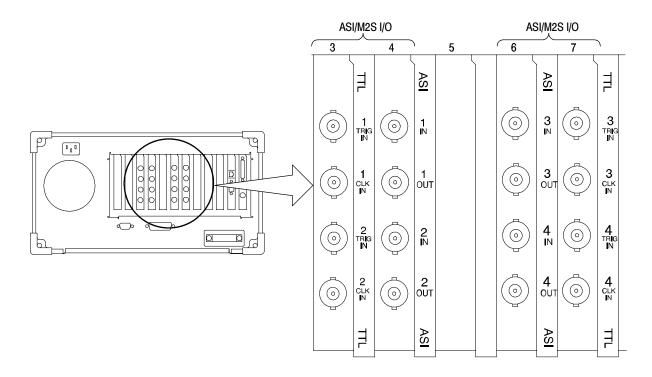
Figure 2-5: Rear-panel configuration with two ASI/M2S (Option AS) interfaces installed
