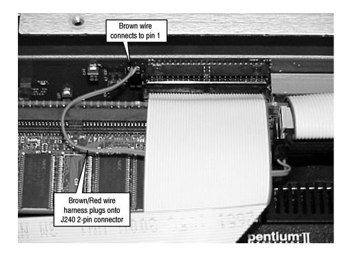
Figure 6-44: Top connection to Controller board
