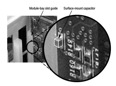
Figure 6-15: Easily damaged capacitor on the PIA+ module
