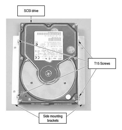
3. Install the mounting brackets on the SCSI drive (see Figure 6-49).
