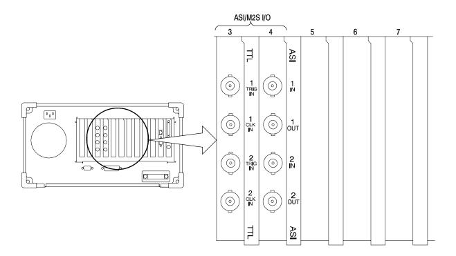
Figure 2-4: Rear-panel configuration with one ASI/M2S (Option AS) interface installed
