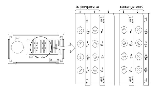
Figure 2-10: Rear-panel configuration with two SSI (Option SS) interfaces installed
