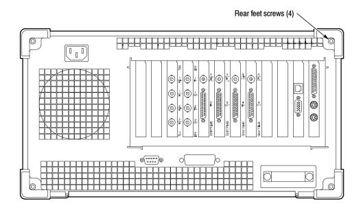
Figure 4-2: Removing the rear-panel feet
