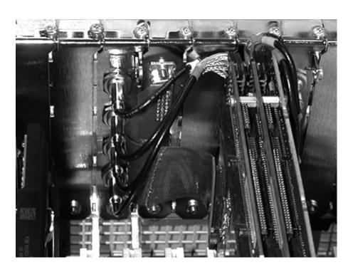
Figure 6-22: Installing the ribbon cable on the DHEI board
