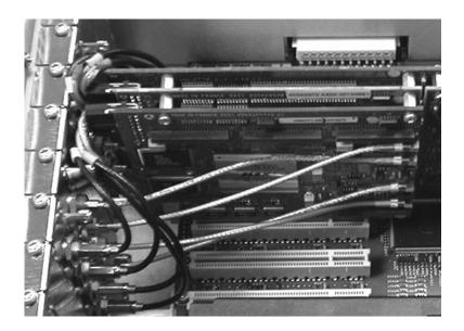
Figure 6-20: Additional ASI or SSI interface installation
