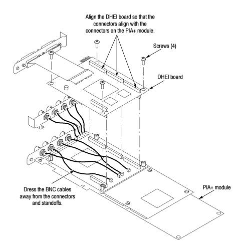
Figure 6-21: Installing the DHEI board on the PIA+ module
