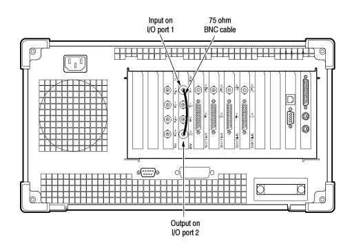
Figure 2-24: Initial setup for the tutorial
