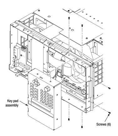
Figure 6-29: Keypad assembly removal
