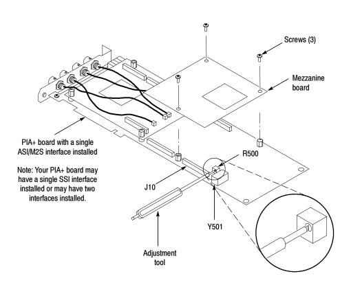
Figure 4-6: Adjusting the 10 MHz reference clock
