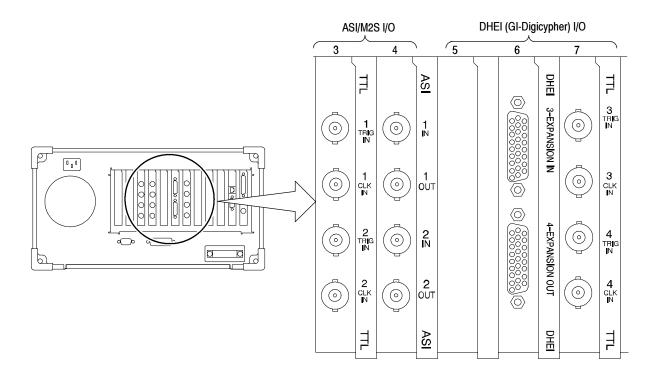
Figure 2-7: Rear-panel configuration with ASI/M2S (Option AS) and DHEI (Option DE) interfaces installed
